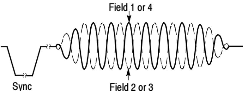
12. If the oscilloscope is triggering on field 2, repeatedly push the **SINGLE SEQ** button until the colorburst waveform changes to the correct phase for field 1, and then push the **RUN/STOP** button to resume triggering the oscilloscope.
