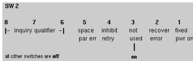
Figure 4-2 Kennedy Dipswitch Bank 2
