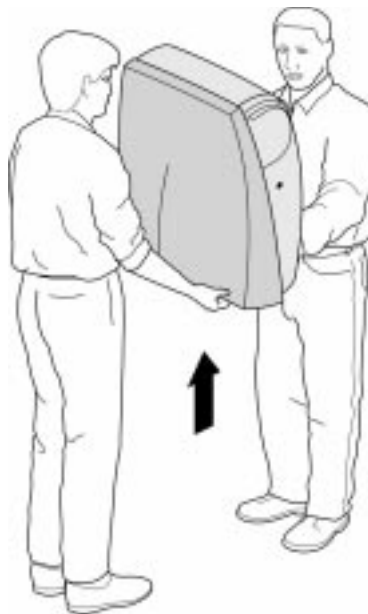
Figure 1-2 Lifting a Silicon Graphics 540 Visual Workstation
