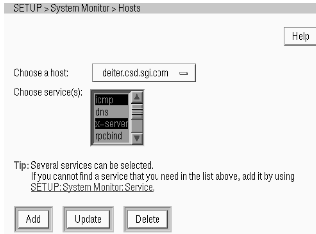
Figure 8-59 Specifying the Services to Monitor on a Host System
