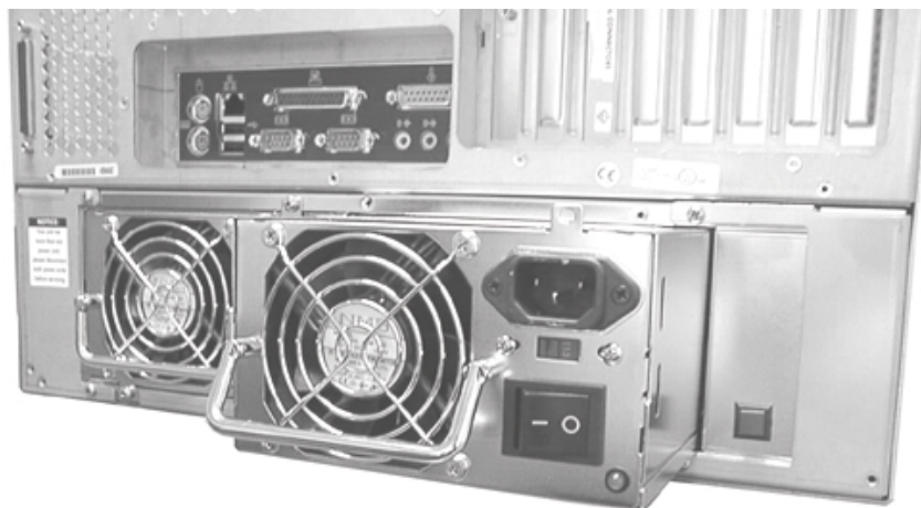
Figure 9-15 Removing or Replacing the Power Supply
