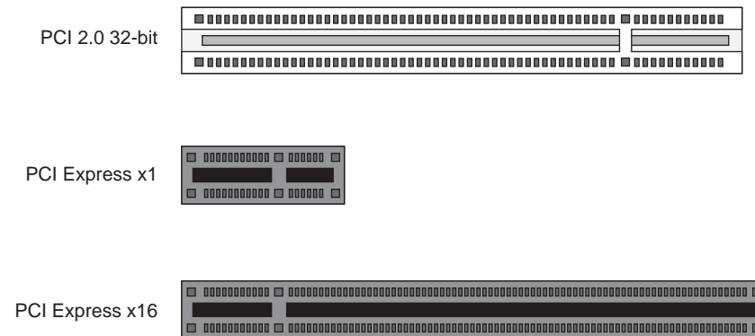
Figure 7-8 Comparison of PCI/PCI-X Connector with PCI Express Connectors
