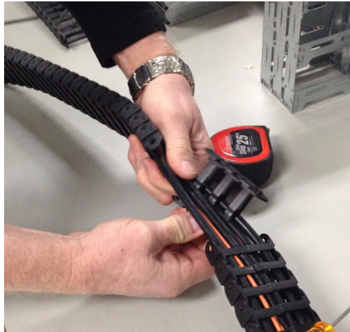
Figure 5-14 Removing the Segment from the Cables
