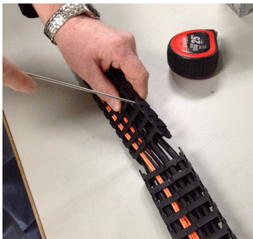
Figure 5-13 Pry Apart the Joint at the Other End
