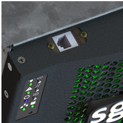
Figure 3-43 MIS-S9D Proprietary Network Interface
