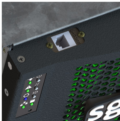
Figure 4-1 MIS-S9D Proprietary Network Interface
