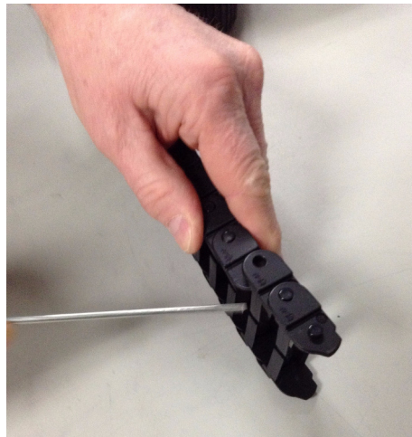
Figure 5-7 Pry the Joint Apart
