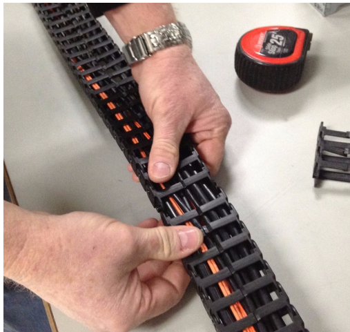
Figure 5-15 Join the Spliced Ends of the Cable Management Arm
