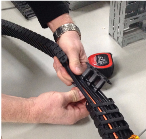
Figure 5-14 Removing the Segment from the Cables
