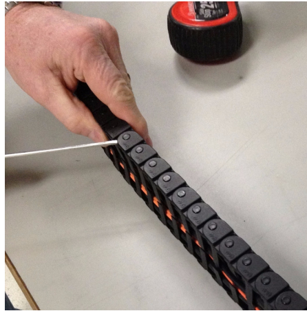
Figure 5-10 Remove Segments from the Middle of a Full Arm
