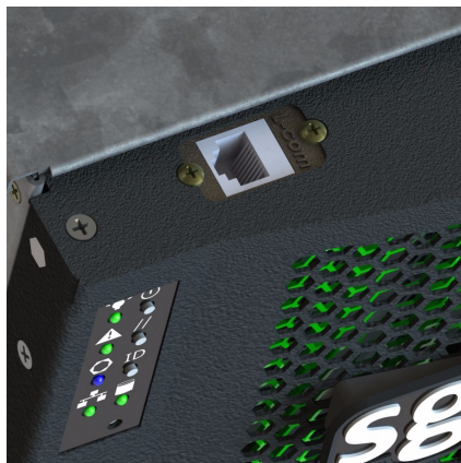
Figure 2-14 MIS-S9D Proprietary Network Interface
