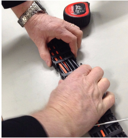
Figure 5-12 Pull Apart the Cable Management Arm
