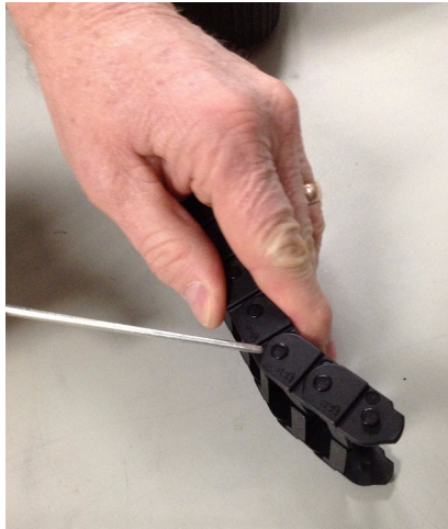
Figure 5-6 Remove Segments from the End of an Empty Arm
