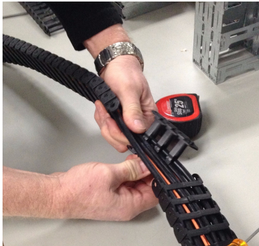
Figure 5-14 Removing the Segment from the Cables
