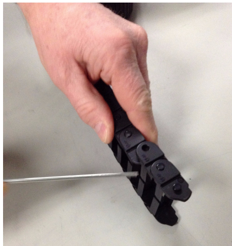
Figure 5-7 Pry the Joint Apart
