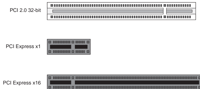
Figure 6-1 Comparison of PCI/PCI-X Connector with PCI Express Connectors
