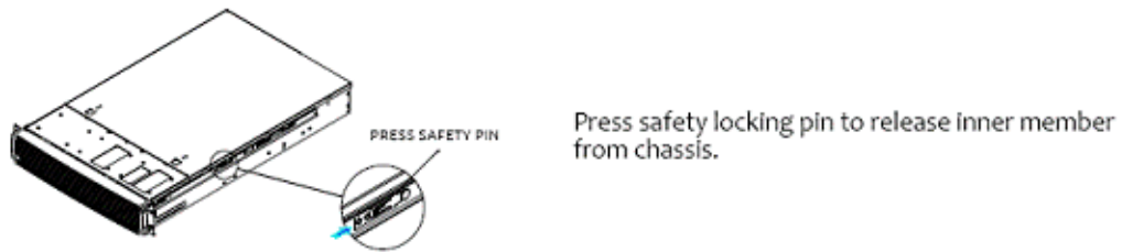
Figure 4-17 Removing the Inner Member from the Chassis
