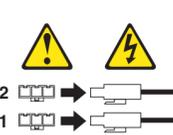
**WARNING (W16) Risk of bodily injury**– Each tray has more than one power cord. To remove all electrical current from the devices, make sure that all of the power cords are disconnected from the power source and that the two-pole 20-amp circuit breaker for the storage array has been disconnected.
