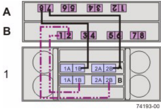
Figure 21 One CE7922 Controller Tray or CE7900 Controller Tray and Two DE6900 Drive Trays with Drive-Side Trunking
