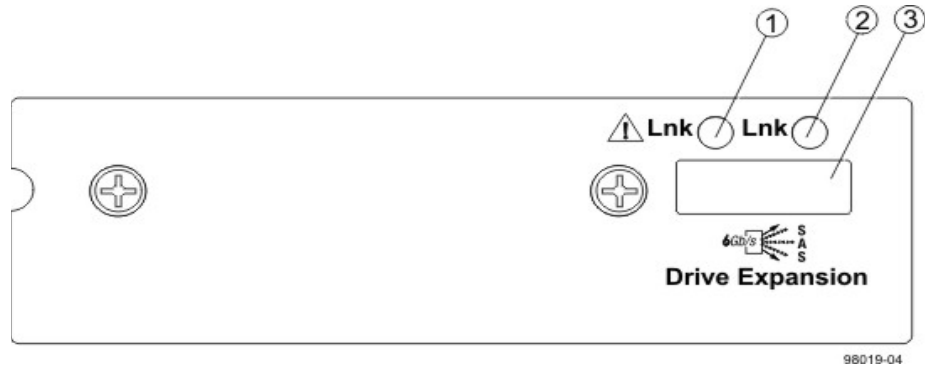
Figure 17 E2600 Right-Rear Subplate with No Host Interface Card
