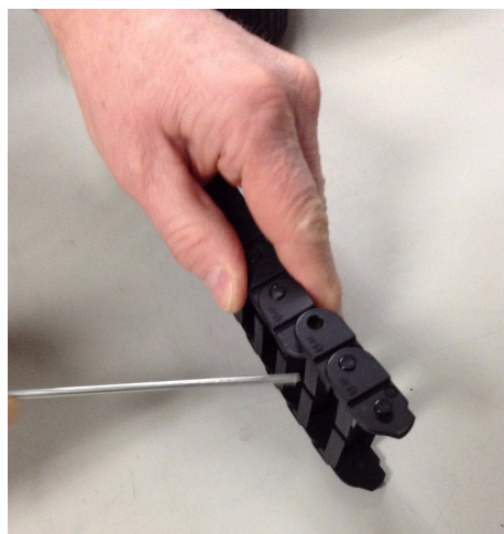
Figure 5-6 Pry the Joint Apart
