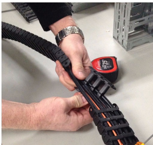
Figure 5-13 Removing the Segment from the Cables
