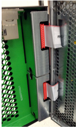
Figure 4-10 Control Panel Ribbon Cables Attached to Front Bezel
