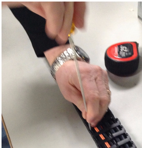
Figure 5-10 Pry Open the Segment Joint
